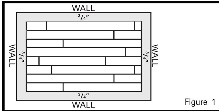
Install layer of 15lb. Builder's felt, overlapped 4" at the seams on top of the wood subfloor. After applying the felt, chalk joists locations for reference when nailing.
