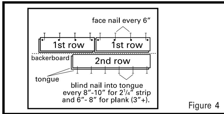
Face nail boards only as required with 7d or 8d finish nails or cleats, ½" from groove, pre-drilling the nail holes to prevent splitting. Countersink nails and fill holes with appropriate wood putty. Nailing schedule is the same as with blind fasteners.
